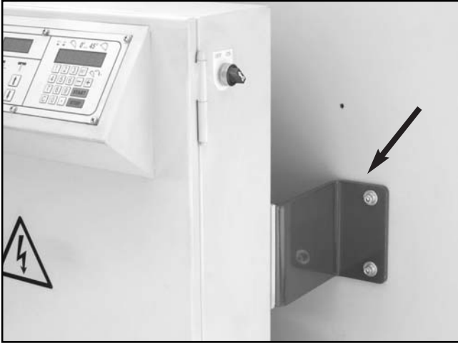
Figure 21. Control panel shipping brace.
